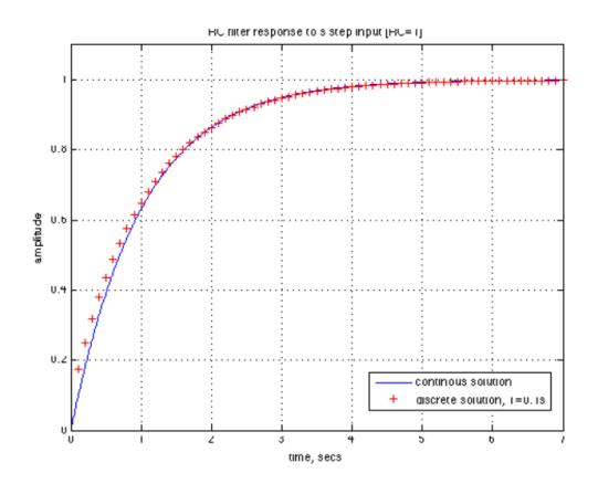
Figure 5.5: Output from an RC-filter for a step function input (RC = Solid line is the analytic solution, crosses indicate discrete solution w timestep of 0.1s
