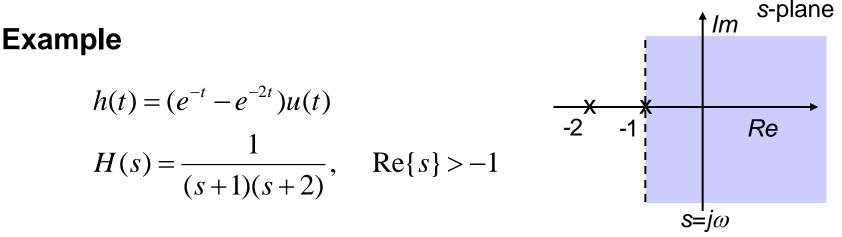
Note that the poles of *H*(*s*) correspond to the powers of the exponential response in the time domain. If the real part is negative, they exponential responses decay => stability. Also, the Fourier transform will exist and the imaginary axis lies in the ROC
